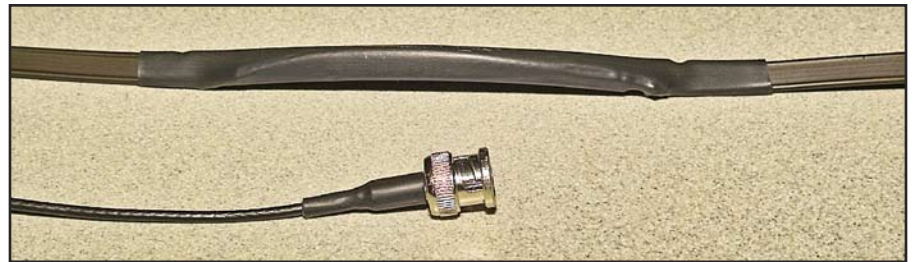
Figure 5 — The \lambda/4 UHF decoupling stub made of RG-174A, covered with heat shrink tubing. This is shown next to the BNC connector that goes to the transceiver.
